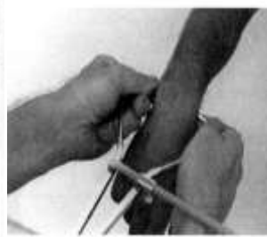
Figure 22 Spreading caliper in place for wrist breadth measurement
